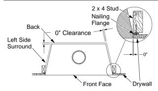
Figure 3 - Minimum Clearances (Top View)
